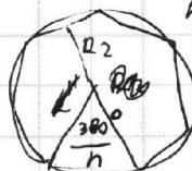
$$\begin{aligned} b &= 2R_2 \tan \frac{180^\circ}{n} \\ c &= 2R_3 \tan \frac{180^\circ}{n} \end{aligned}$$
